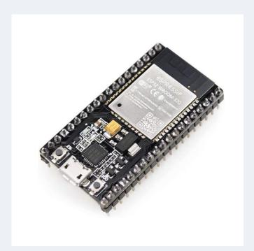
He educated us that the ESP32 is in fact a much more powerful micro controller. It has a speed of 240MHz compared to Arduino Uno 16MHz. It also has built in WiFi and Bluetooth which is perfect for our intention.
